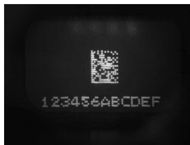
Continuous Ink Jet (CIJ) direct on products
