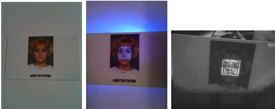
A select example of successful print behind a readable UV fluorescing bar code
